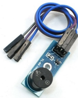
Figure 15: 9012 Transistor Driver Buzzer
