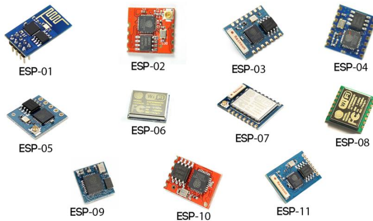
Figure 1 The ESP8266 is available in various module configuration [1]. The main difference is the selection of pinouts from the chip.
