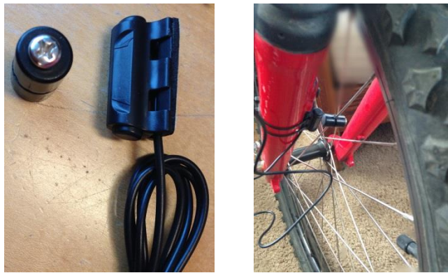
Figure 8 – The Detailed Position of Magnet & Magnetic Sensor
