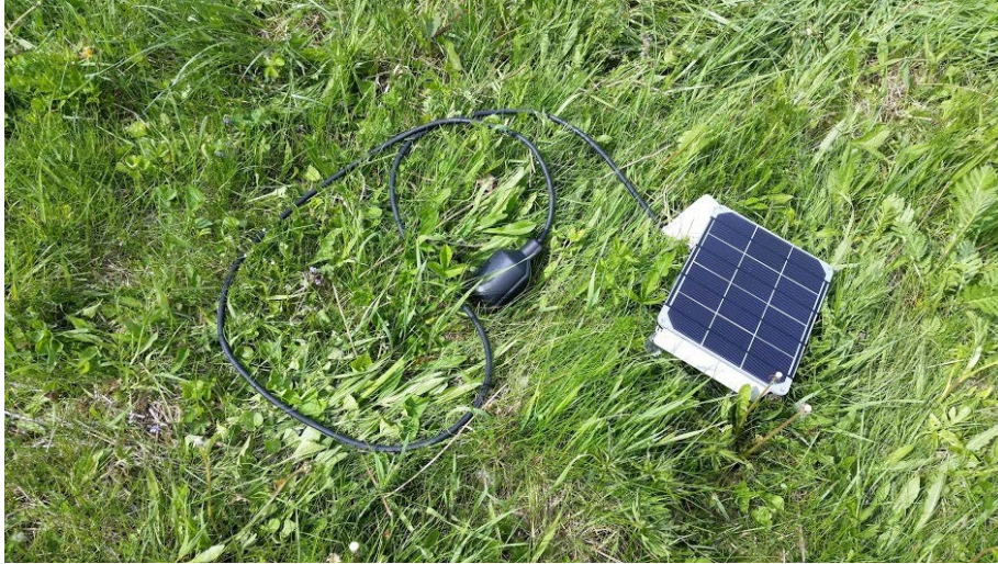
Figure 10: Final assembly of tank-side panel and float switch
