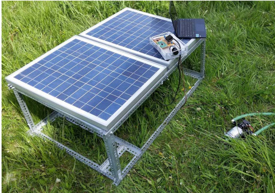
Figure 11: Final assembly of pump-side panel, circuit, and motor (opaque half of box removed for visual).
