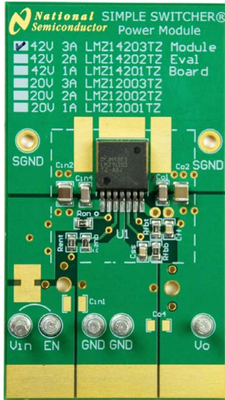
Figure 4: National Semiconductor (Acquired by Texas Instruments) LMZ14201 evaluation board. This is a picture of the 3A model, but the 1A model looks virtually identical. (ti.com)
