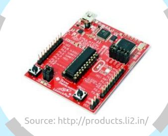
MSP430 generates 3.3V 2kHz 5-95% duty sweep test signal
