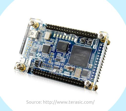
Cyclone IV is "CPU" of the system: data acquisition, hardware triggering, PSU control, signal generator, logic analyzer
