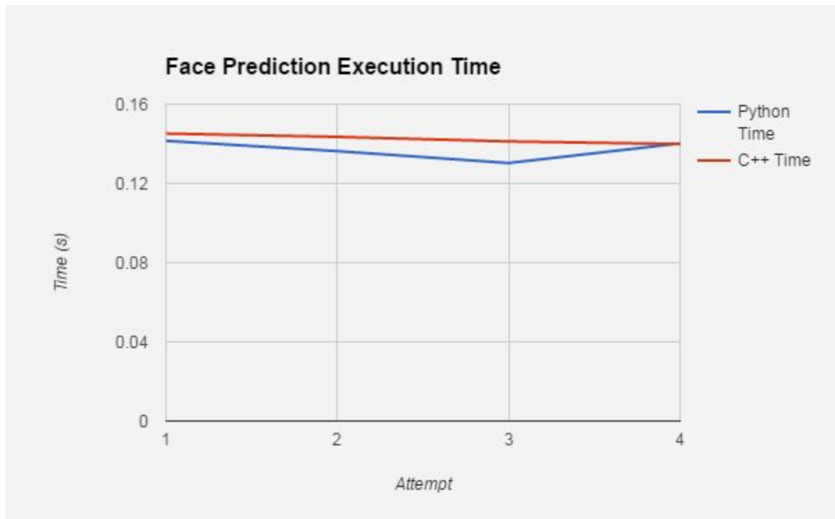
Figure 27: Execution time for prediction algorithm for Python and C++ implementations.
