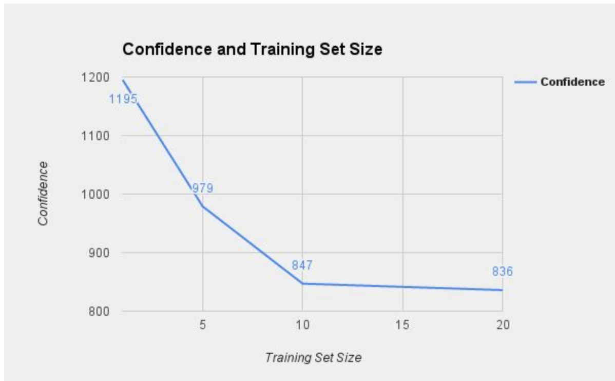
Figure 22: Results testing the confidence value vs. the number of positive training images used.
