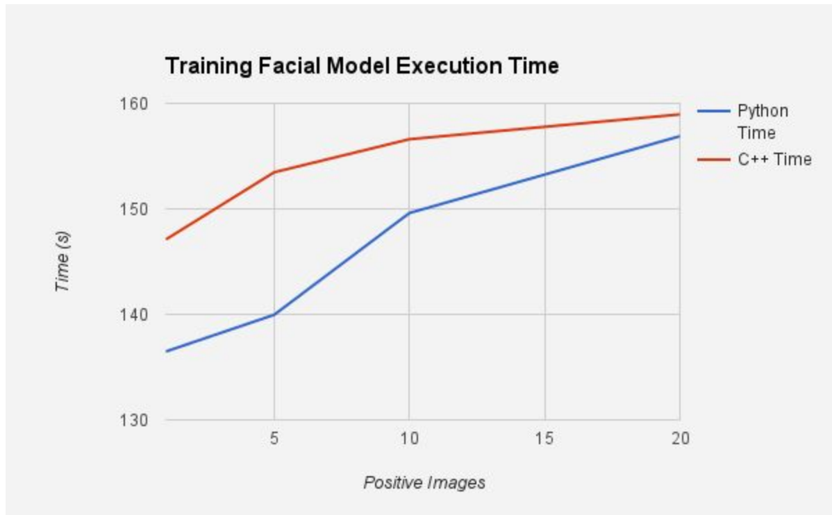
Figure 24: Graph comparing the time to train the facial model versus the number of images used for Python and C++ implementations.
