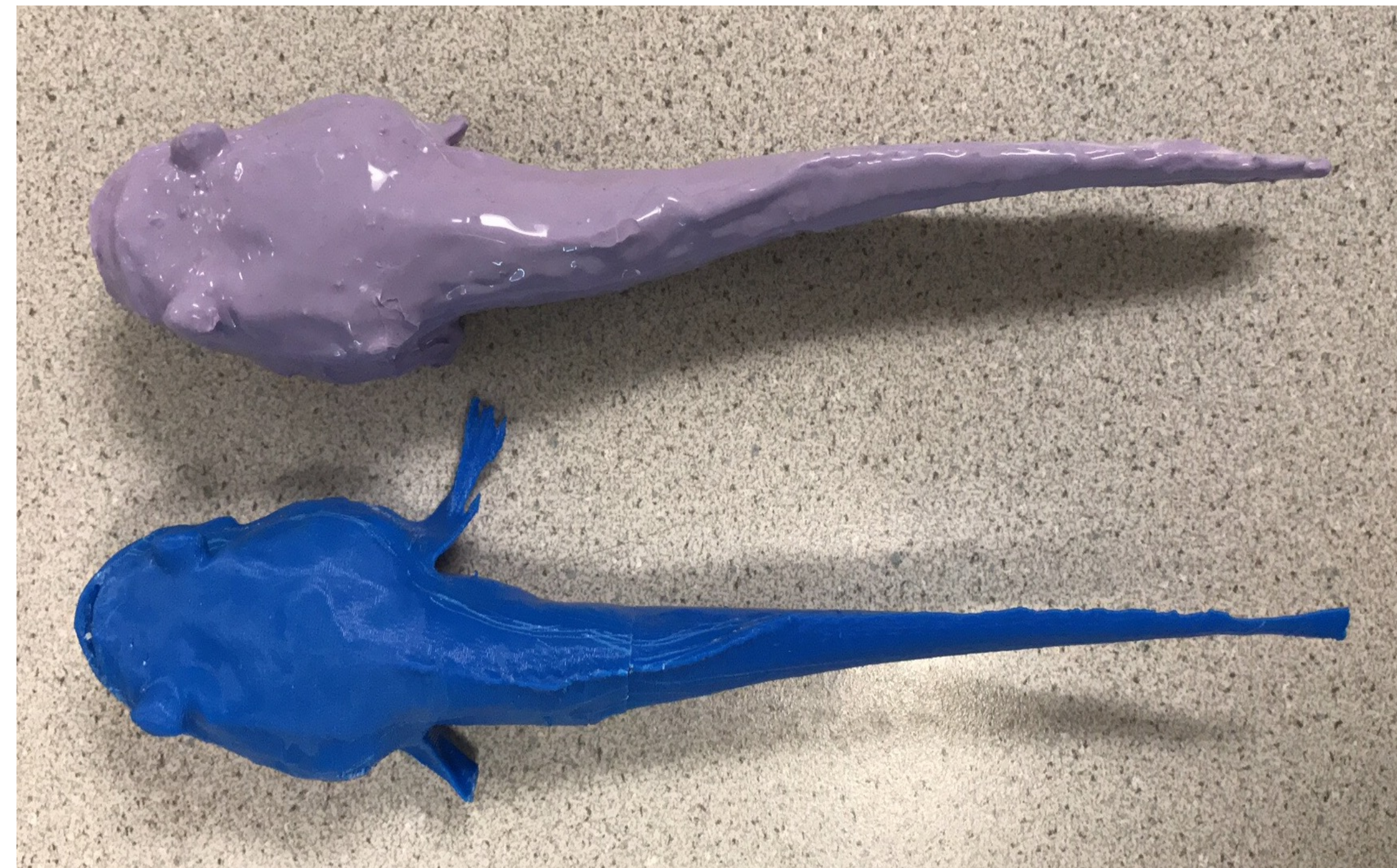
Figure 2. 3D printed (lower) and silicon casted (upper) fish models. The accuracy of the fish model is around 90% in dimensions, and enough details, such as dorsal fin and pectoral fins are presented.
