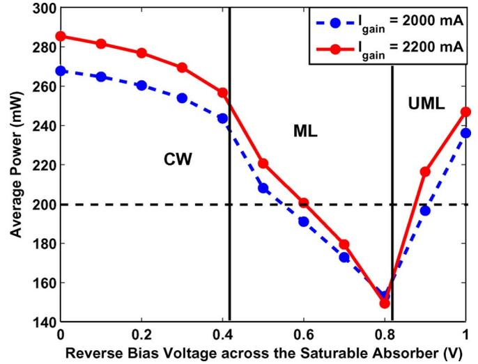
Fig. 3. Measured average optical power as a function of the reverse bias voltage across the saturable absorber for two different gain currents. CW, ML, and UML indicates continuous wave, mode-locked, and unstable mode-locked operations, respectively.
