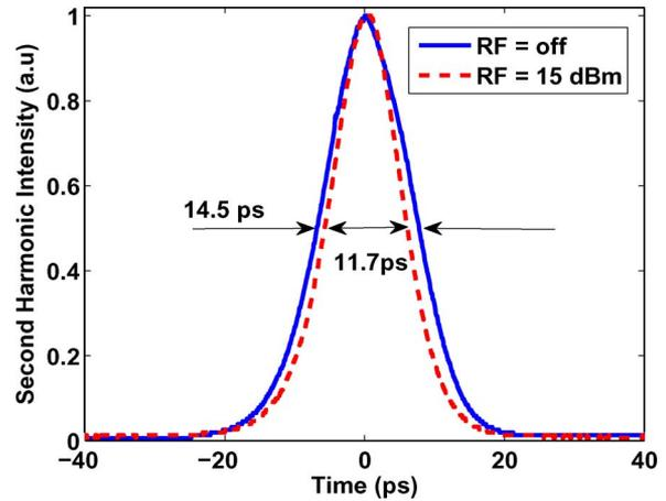
Fig. 4. Measured pulse intensity autocorrelation. The extracted pulsewidths in the absence and presence of the RF signal are indicated. The pulsewidth is reduced slightly when the RF signal is switched ON. The gain current is 1000 mA and the reverse bias voltage across the saturable absorber is 0.8 V.
