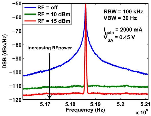
Fig. 2. Double sideband (DSB) noise spectrum for hybrid mode-locking for an average power  $>200$  mW. Increasing the applied RF power results in a reduction in the measured noise.
