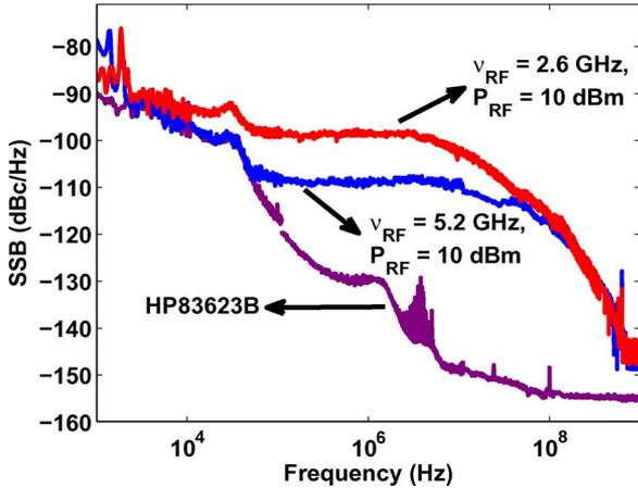
Fig. 6. Applying a 2.6-GHz external RF signal results in subharmonic hybrid mode-locking. The SSB phase noise shows an increase in the timing noise compared to the case of fundamental hybrid mode-locked operation. The gain current was 1000 mA and the reverse bias voltage was 0.3 V.
