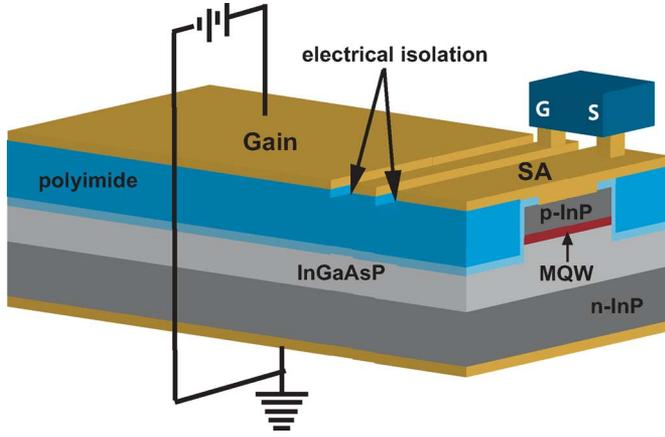
Fig. 1. Schematic of the cross section of the laser. The mode resides mainly in the InGaAsP waveguide layer. The figure also shows the scheme used to reverse bias the saturable absorber (SA) section using a G-S probe.
