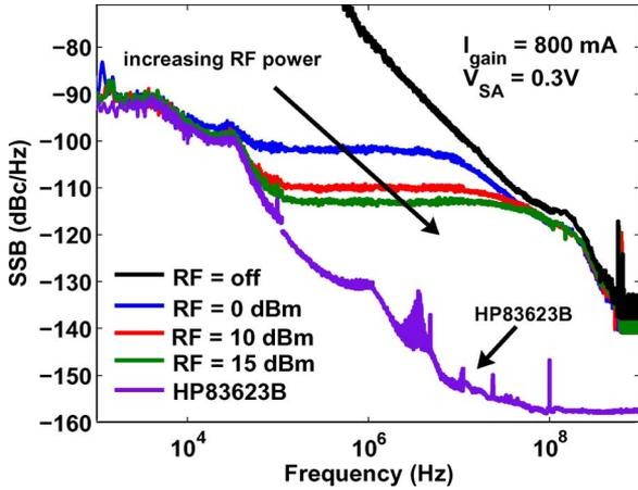
Fig. 5. SSB phase noise for various applied RF powers. Also seen in the plot is the SSB for the case when the RF signal is switched OFF (passive mode-locking). The SSB for the RF source shows that beyond 50 kHz, the timing noise is mainly due to the laser.
