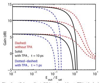
Fig. 2. (Color online) SOA gain without TPA (dashed curves) and with TPA assuming FWHM pulse widths of 10 ps (solid curves) and 1 ps (dotted–dashed curves). The SOA parameters are given in the text and correspond to the InGaAsP SOA in [3].  $E_{\rm sat}$ =100 pJ. In each case, the three curves correspond to unsaturated material gain values ( $g_o$ ) of 800, 1200, and 1600 cm<sup>-1</sup>.
