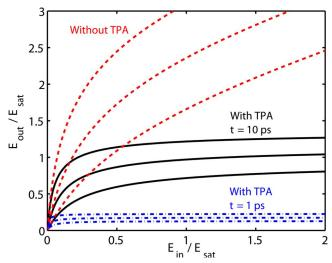
Fig. 1. (Color online)  $E_{\rm out}$  versus  $E_{\rm in}$  curves without TPA (dashed curve) and with TPA assuming FWHM pulse widths of 10 ps (solid curve) and 1 ps (dashed–dotted curve). The SOA parameters are given in the text and correspond to the InGaAsP SOA in [3].  $E_{\rm sat}$ =100 pJ. In each case, the three curves correspond to unsaturated material gain values ( $g_o$ ) of 800, 1200, and 1600 cm<sup>-1</sup>.
