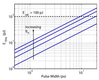
Fig. 3. (Color online) Values of  $E_{\rm TPA}$  are plotted as a function of the FWHM pulse width  $\tau$ . The SOA parameters are the same as in Figs. 1 and 2. The four curves correspond to unsaturated material gain values  $(g_o)$  of 400, 800, 1200, and 1600 cm<sup>-1</sup>.
