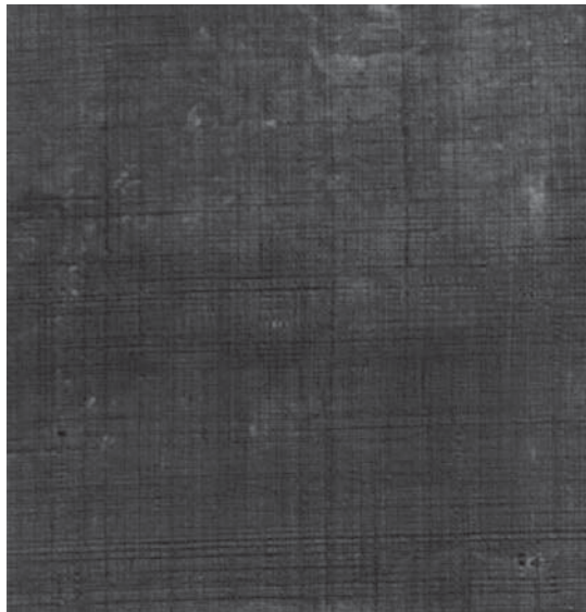
Figure 1. Thread count or density is determined by counting the number of warp and weft threads in a predetermined square area using an X-radiograph. It can be measured by humans or by computerized image/signal processing.
