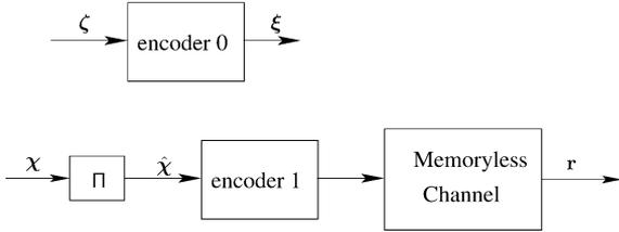
Fig. 6. The system which the serial turbo decoder assumes.
