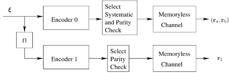
Fig. 1. Parallel concatenation of two convolutional codes with interleavers.
