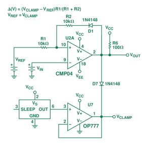
Figure 8. Precision clamp circuit.
