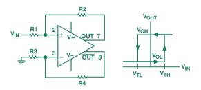
Figure 7. Single-supply comparator with bipolar input.
