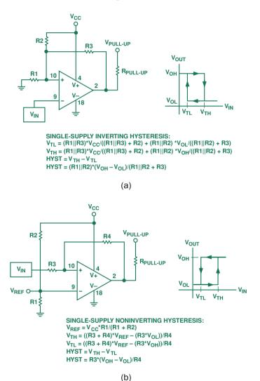
Figure 5. Comparators in single-supply operation.
