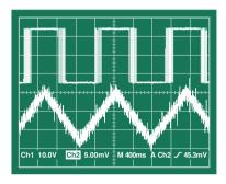
Figure 1. Noise causes multiple transitions.
