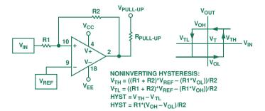
Figure 4. Comparator using noninverting input, dual supplies.
