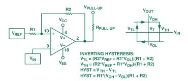
Figure 3. Comparator using inverting input, dual supplies.
