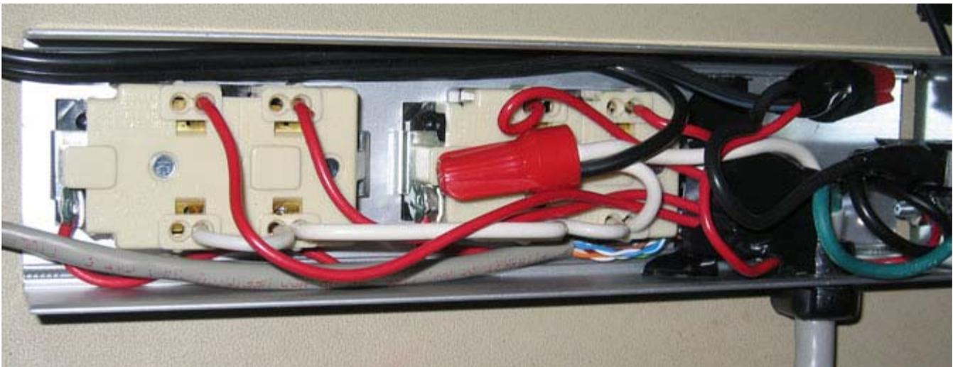
Here's the inside of the strip right before being closed up. There used to be a small switching plug jammed in there too, but somehow it blew up. So, instead there's a wire coming out that hooks up to the power supply. The relays are covered with electrical tape, right next to the main wire bundle. Interestingly, the earth ground wires of the outlets weren't initially hooked to anything, but we fixed that.
