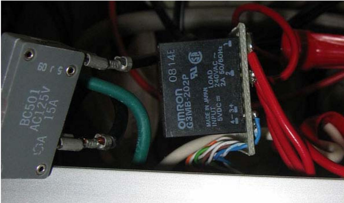
The circuit breaker on the left protected the rest of the world in case something within the box's relays on the right were hooked to the microcontroller with Cat5 twisted pair cable, and to the other gauge stranded wire.
