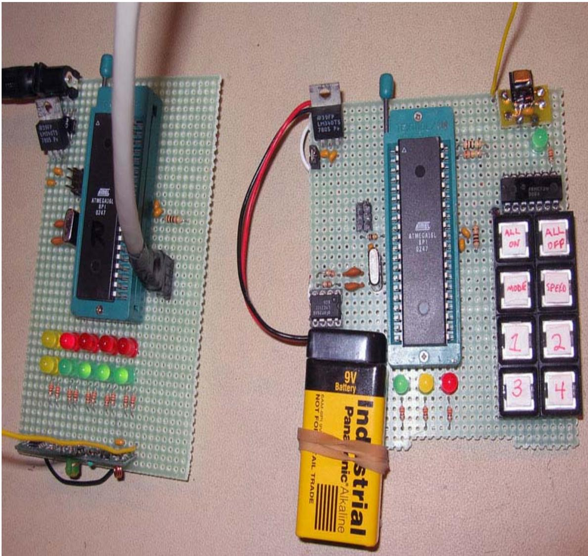
Here are the two circuit boards, transmitter on right and receiver on left. Both used a 17cm pier antenna.
