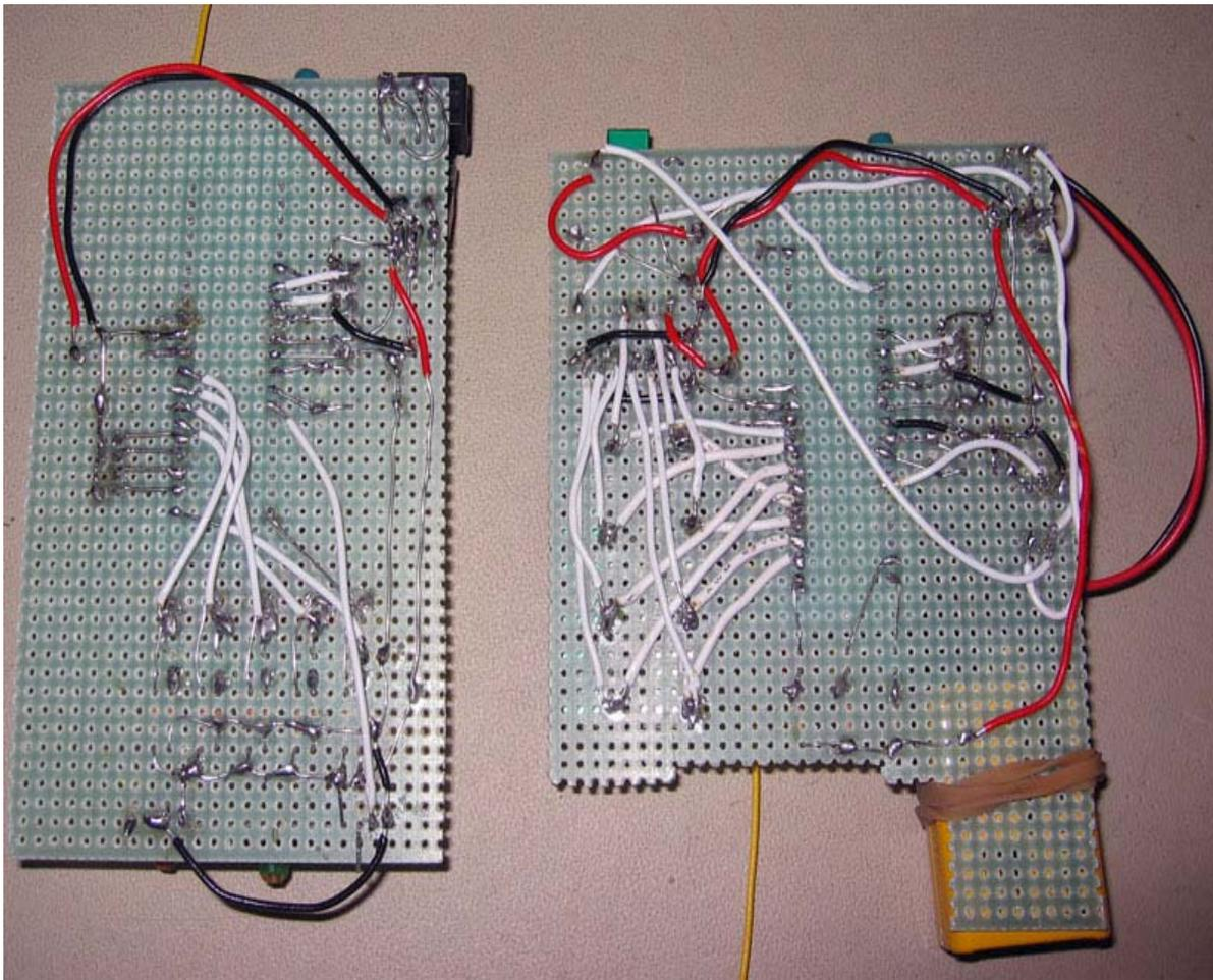
This is the bottom of the two boards. Soldering these two boards was rather tedious and difficult. The connections are solid and the wires aren't going anywhere. The only real way to neaten it up is printed circuit boards, but that's a little advanced for this early prototyping stage.
