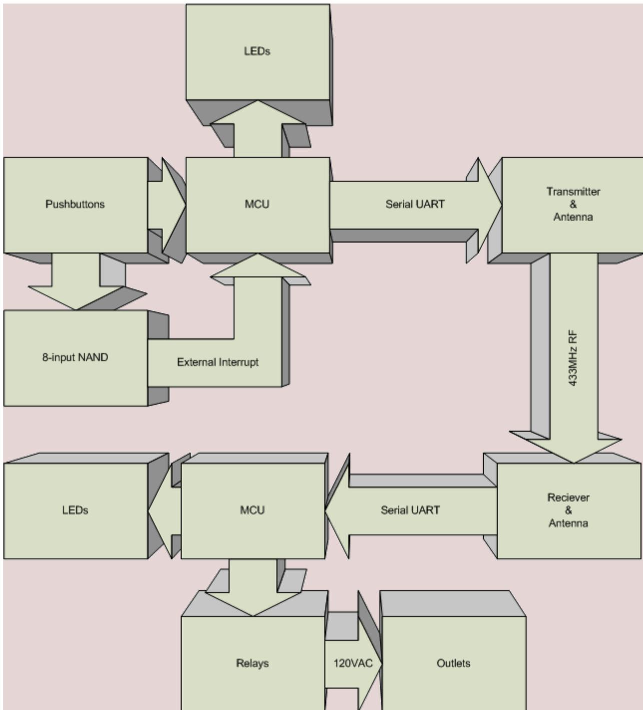
The transmitter is normally in a power-down sleep state, to conserve battery life. All components were selected to have low-quiescent current, to minimize the power wasted when nothing is happening. The pushbuttons cause an external interrupt, which wakes up the MCU, and reads the port. It then sends the port state through the UART to the RF transmitter if only one button was pressed. This makes detecting data errors simpler, since the data byte must have seven 1s and one 0.
