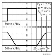
Inverting Small Signal Pulse Response at 5V
