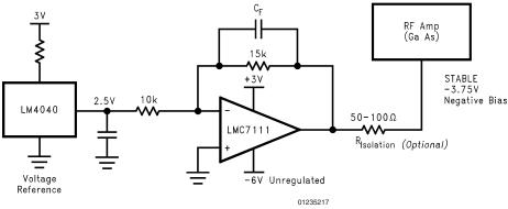
$C_{\mbox{\scriptsize F}}$  and  $R_{\mbox{\scriptsize isolation}}$  prevent oscillations when driving capacitive loads.
