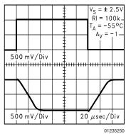
Inverting Large Signal Pulse Response at 5V
