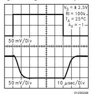
Inverting Large Signal Pulse Response at 5V
