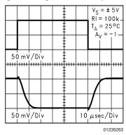
**Inverting Large Signal Pulse Response at 10V**
