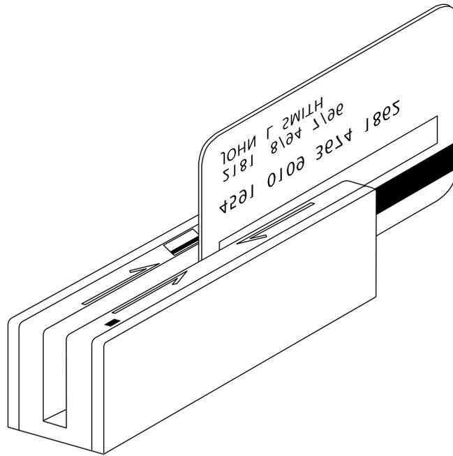
**Figure 1-1. Port-Powered Swipe Reader**
