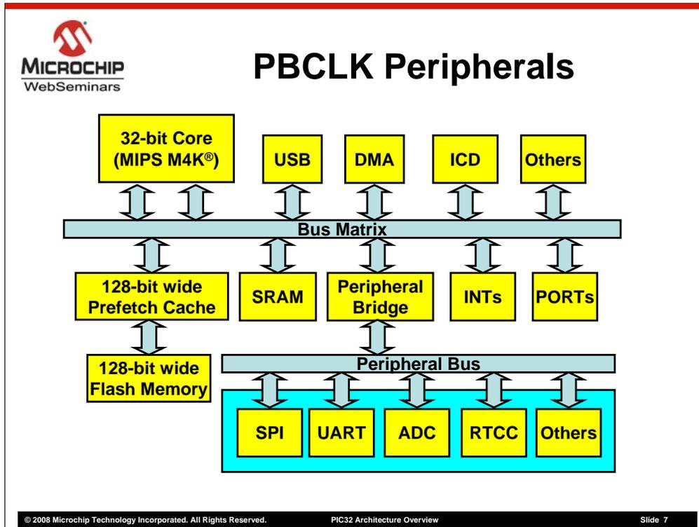
The PBCLK Peripherals are one more class of peripherals. These peripherals run from PBCLK. The SPI, UART, ADC, RTCC, I2C, etc., are examples of the PBCLK peripherals. The exact value of the PBCLK is determined by the setting of the Peripheral bridge module. Available options are to run PBCLK at 1:1, 1:2, 1:4 and 1:8 of SYSCLK speed. Normally, PBCLK peripherals are slow in speed and do not require very high data throughput.
