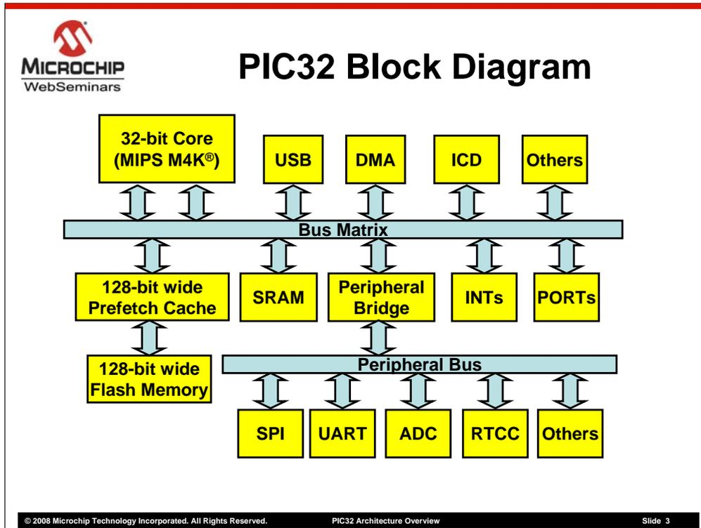
This is a simplified view of the PIC32 chip. The PIC32 employs the M4K<sup>®</sup> 32-bit core from MIPS Technologies. The M4K is a Harvard architecture based core. It contains separate Instruction and Data busses connected to the Bus Matrix. I will provide you with more information about M4K in next slide.
