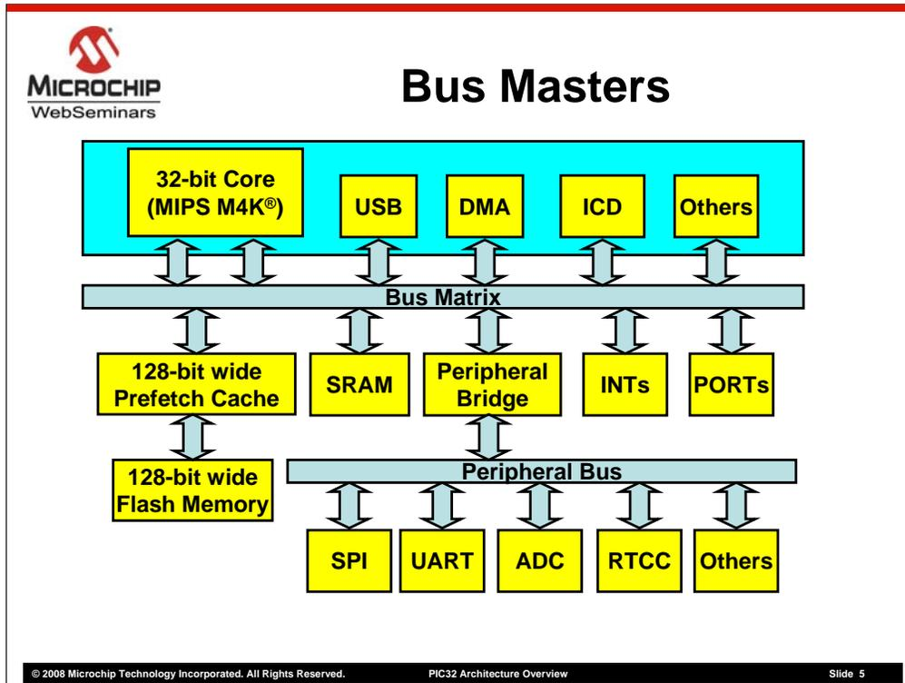
The PIC32 architecture uses a concept called Bus Master modules. The Bus Masters are a special set of modules that can initiate a read or write transaction of other modules called “Targets”. For example, the CPU can read and write to SRAM or any other peripheral. Similarly, the DMA can read and write to any other peripherals on the bus. At present, CPU, ICD, USB, and DMA are the Bus Masters in PIC32 architecture. Future PIC32 products may add more Bus Master modules.
