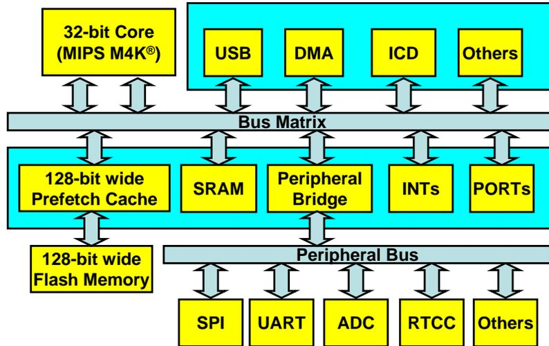
Peripherals such as the Prefetch Cache, USB, DMA, SRAM, Interrupts and I/O PORTs are called SYSClk Peripherals. These peripherals run at the same speed as the CPU and other Bus Masters. As a result, all accesses to the SYSClk peripherals complete in one cycle. Typically peripherals with high data throughput are placed on the SYSClk bus.
