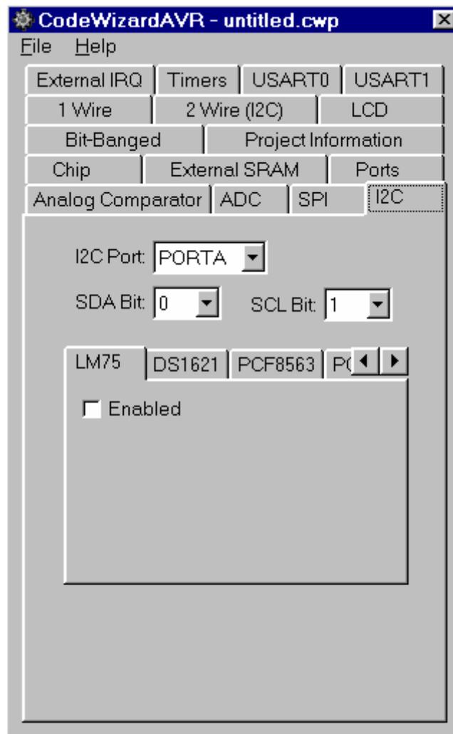
Using the **I<sup>2</sup>C Port** list box you can specify which port is used for the implementation of the I<sup>2</sup>C bus. The **SDA Bit** and **SCL Bit** list boxes allow you to specify which port bits the I<sup>2</sup>C bus uses.
