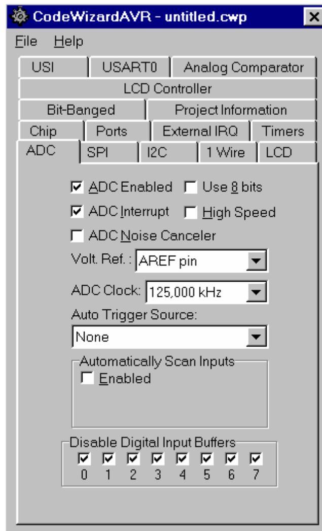
This is accomplished by checking the corresponding **Disable Digital Input Buffers** check boxes. If the **Automatically Scan Inputs** option is enabled, then the corresponding digital input buffers are automatically disabled for the ADC inputs in the scan range.
