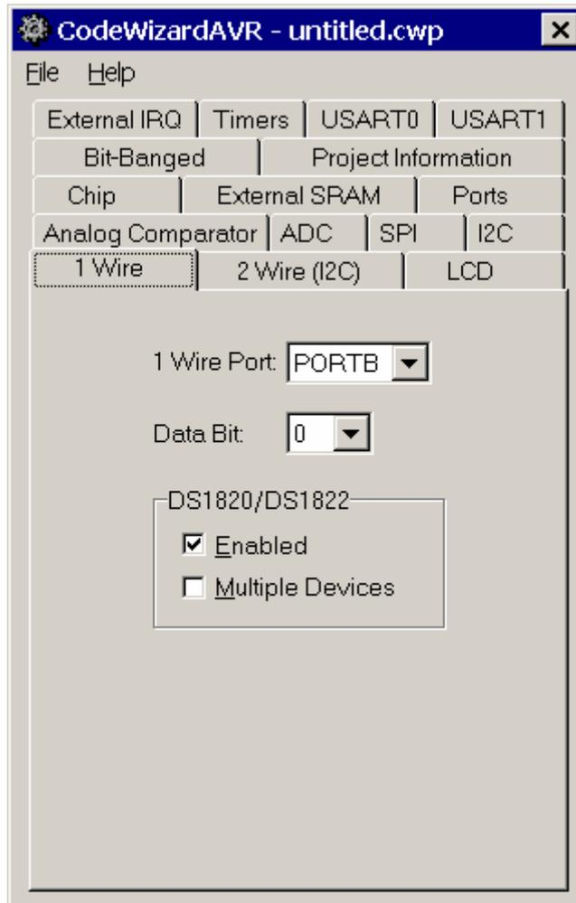
If you use several DS1820/DS18S20 devices connected to the 1 Wire bus, you must check the **Multiple Devices** check box. Maximum 8 DS1820/DS18S20 devices can be connected to the bus. The ROM codes for these devices will be stored in the `ds1820_rom_codes` array.
