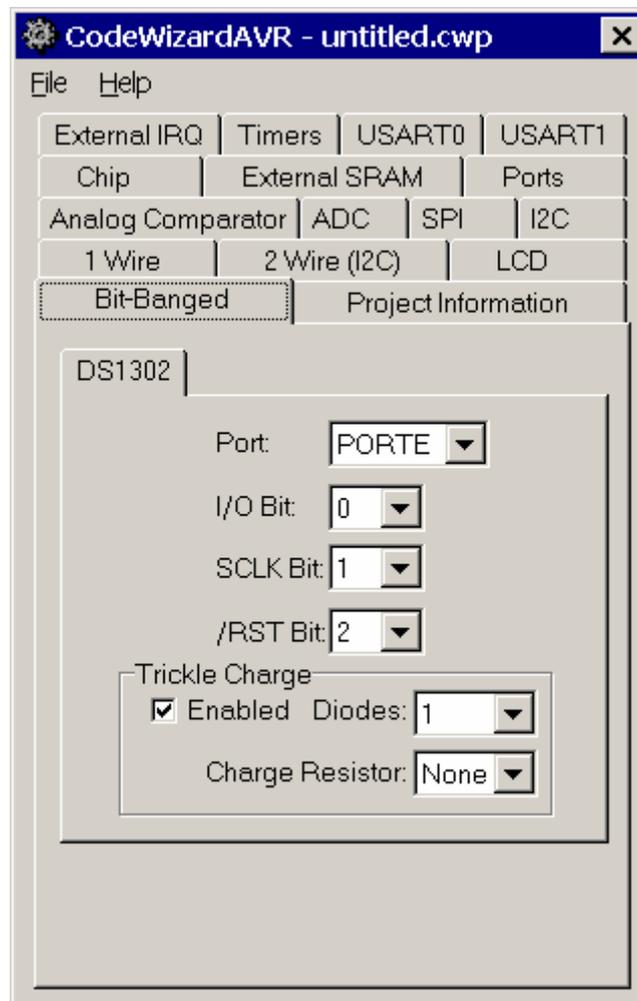
Using the **Port** list box you can specify which port is used for connecting with the DS1302. The **I/O Bit**, **SCLK Bit** and **/RST Bit** list boxes allow you to specify which port bits are used for this. The DS1302's trickle charge function can be activated by checking the **Trickle Charge|Enabled** check box.
