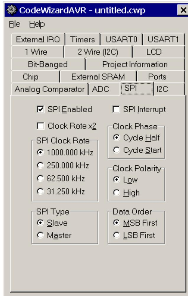
Checking the **SPI Enabled** check box enables the on-chip SPI interface.
