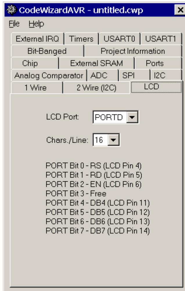
Using the **LCD Port** list box you can specify which port is used for connecting the alphanumeric LCD. The **Chars./Line** list box allows you to specify the number of characters per display line. This value is used by the `lcd_init` function.
