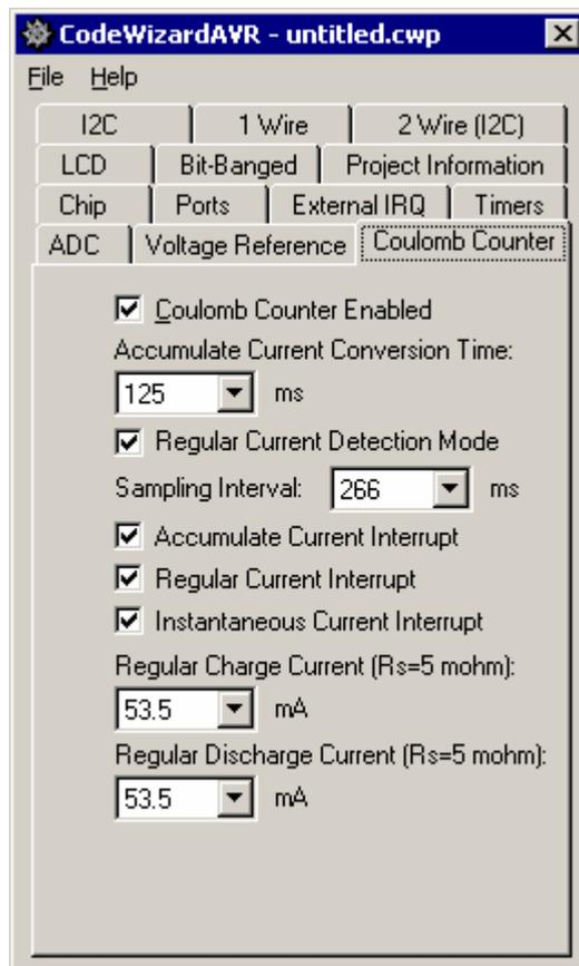
Checking the **Coulomb Counter Enabled** check box enables the Coulomb Counter Sigma-Delta ADC.
