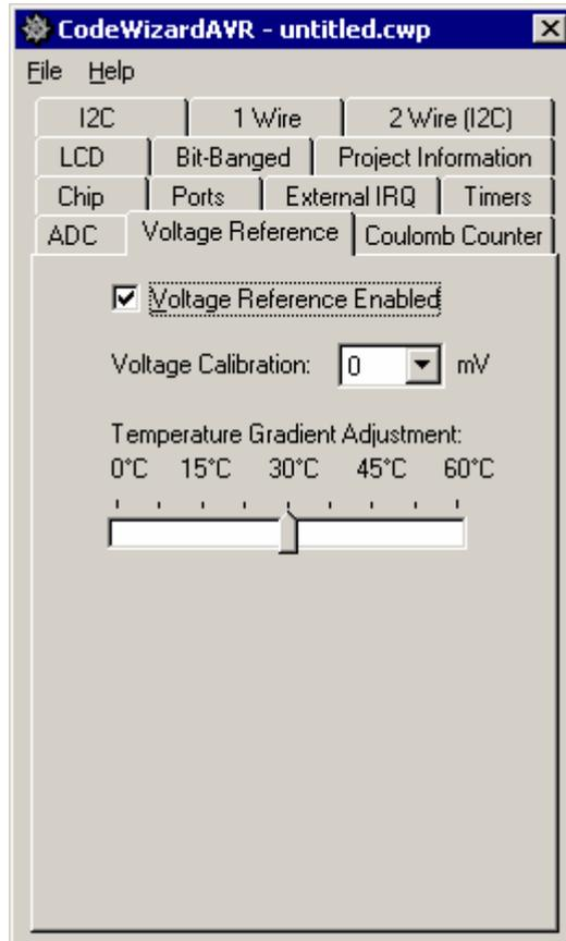
Checking the **Voltage Reference Enabled** check box enables the precision voltage reference. The **Voltage Calibration** list box allows for precision adjustment of the nominal value of the reference voltage in 2mV steps.
