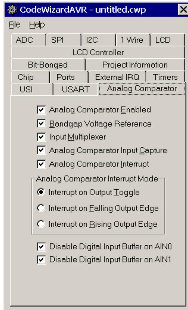
Checking the **Analog Comparator Enabled** check box enables the on-chip analog comparator. Checking the **Bandgap Voltage Reference** check box will connect an internal voltage reference to the analog comparator's positive input.
