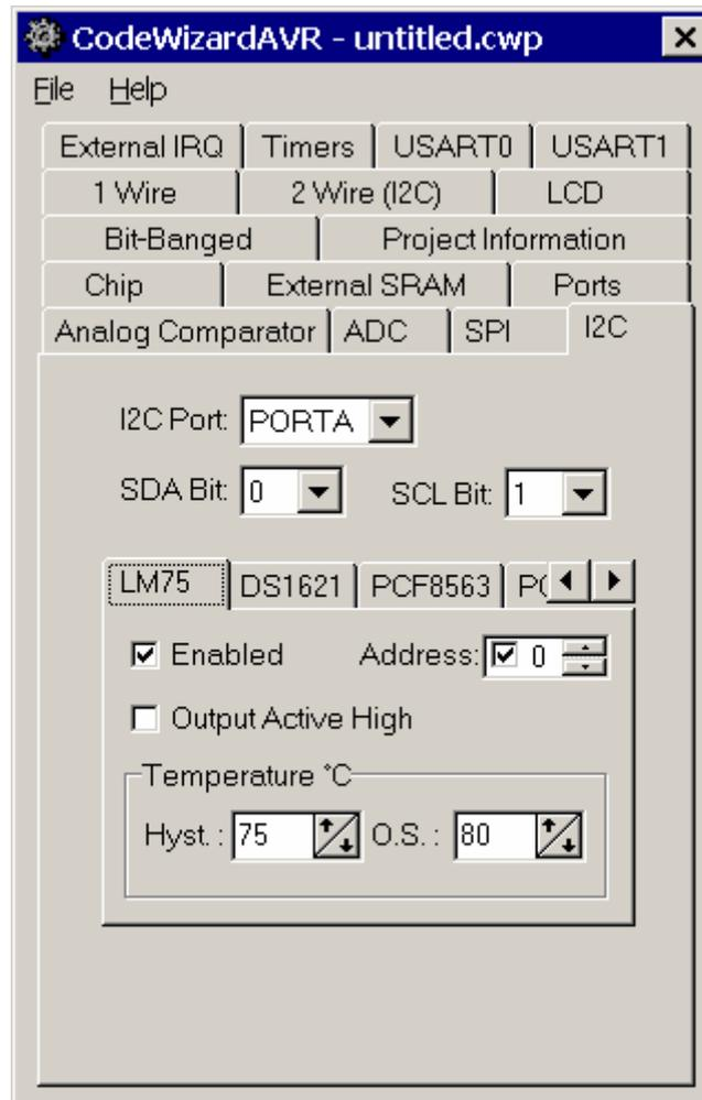
The **LM75 Address** list box allows you to specify the 3 lower bits of the I<sup>2</sup>C addresses of the LM75 devices connected to the bus. Maximum 8 LM75 devices can be used.
