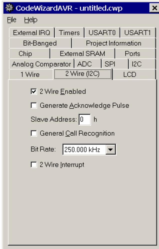
The AVR chip's 2 Wire interface can be enabled by checking the **2 Wire Enabled** check box. If the **Generate Acknowledge Pulse** check box is checked the ACK pulse on the 2 Wire bus is generated if one of the following conditions is met:
