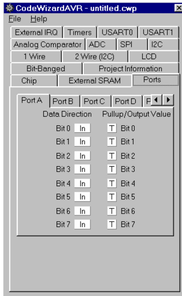
You can choose which port you want to configure by selecting the appropriate **PORT x** tab. By clicking on the corresponding **Data Direction** bit you can set the chip pin to be output (Out) or input (In).
