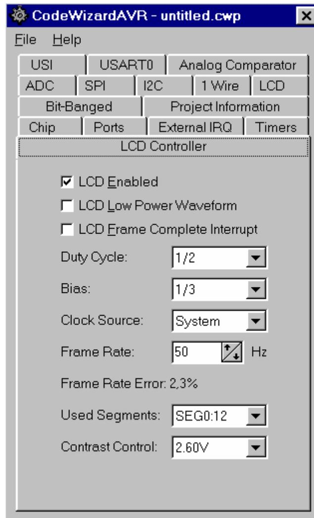
The ATmega169V/L on chip LCD controller can be enabled by checking the **LCD Enabled** check box. By checking the **LCD Low Power Waveform** check box, the low power waveform will be outputted on the LCD pins. This allows reducing the power consumption of the LCD.
