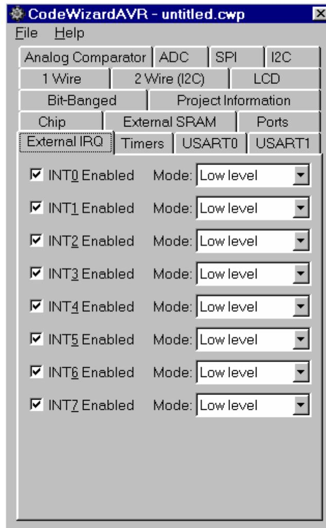
Checking the appropriate **INTx Enabled** check box enables the corresponding external interrupt. If the AVR chip supports this feature, you can select if the interrupt will be edge or level triggered using the corresponding **Mode** list box.
