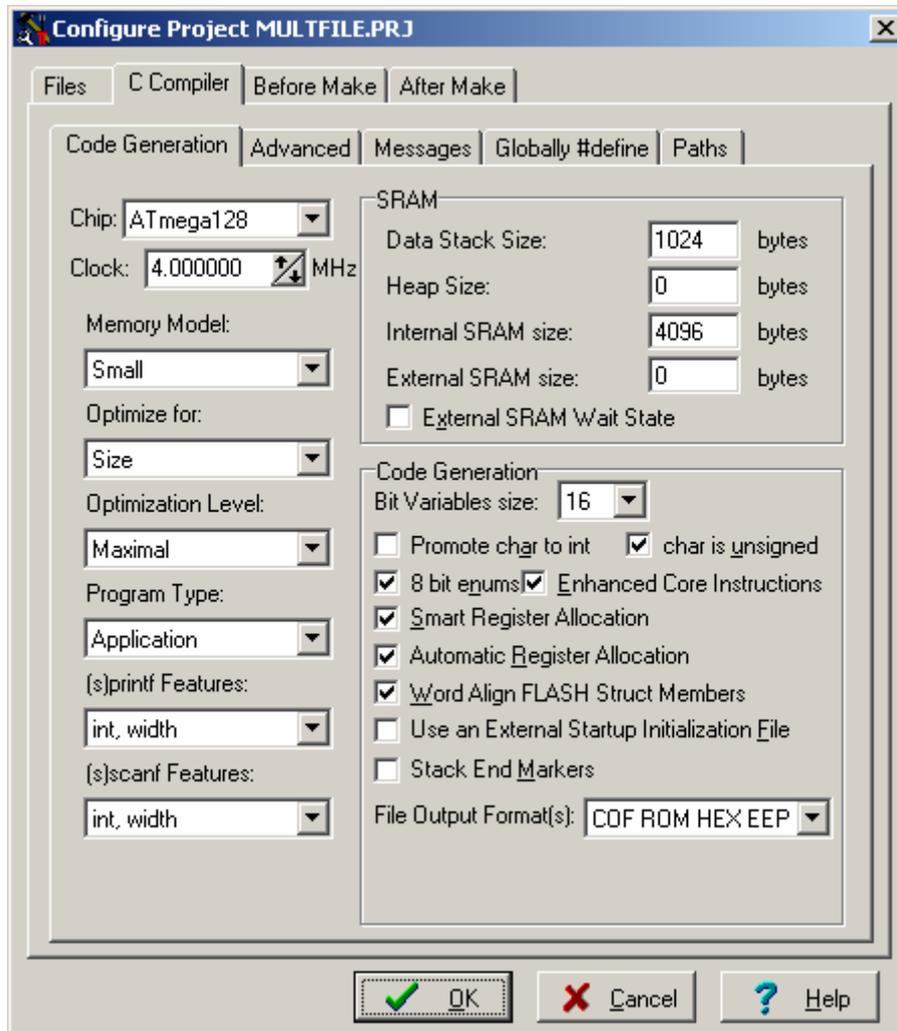
You can select the target AVR microcontroller chip by using the **Chip** combo box. You must also specify the **CPU Clock Frequency** in MHz, which is needed by the Delay Functions, 1 Wire Protocol Functions and Maxim/Dallas Semiconductor DS1820/DS18S20 Temperature Sensors Functions.
