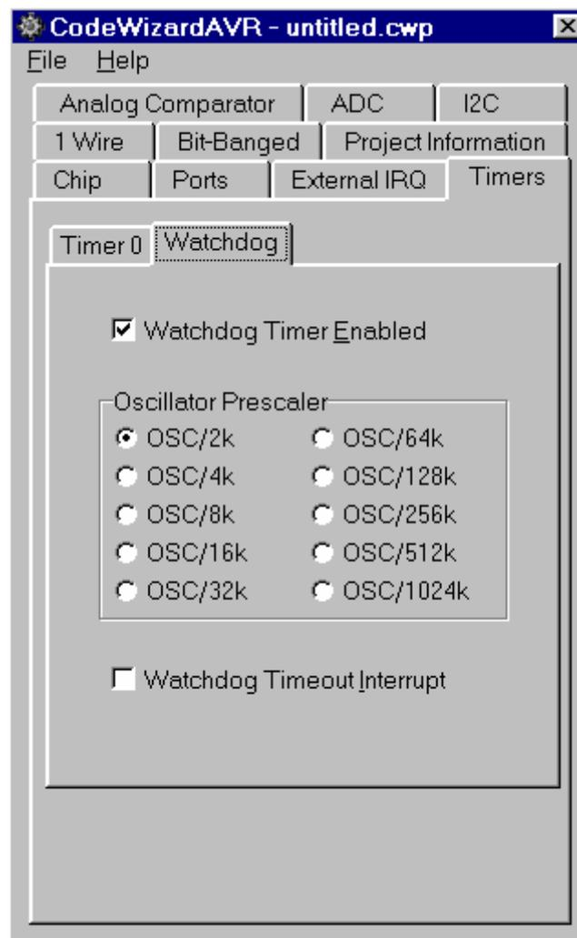
Checking the **Watchdog Timer Enabled** check box activates the watchdog timer.
