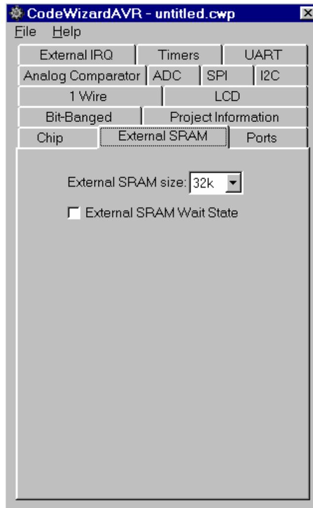
The size of external SRAM can be specified using the **External SRAM Size** list box. Additional wait states in accessing the external SRAM can be inserted by checking the **External SRAM Wait State** check box. The MCUCR register in the startup initialization code is configured automatically according to these settings.
