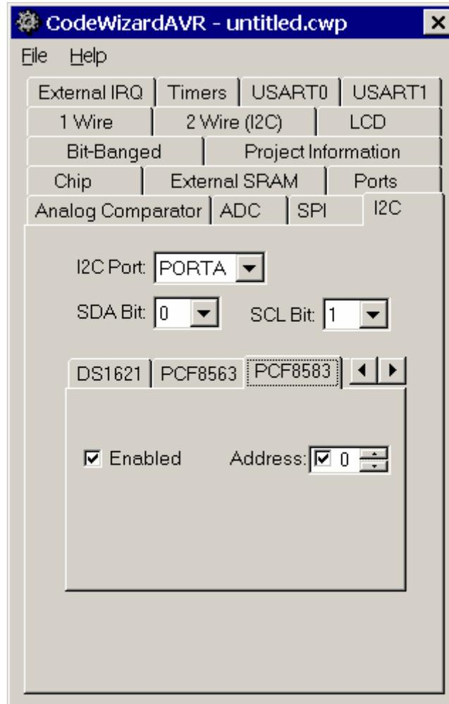
The **PCF8583 Address** list box allows you to specify the low bit of the I<sup>2</sup>C addresses of the PCF8583 devices connected to the bus. Maximum 2 PCF8583 devices can be used.
