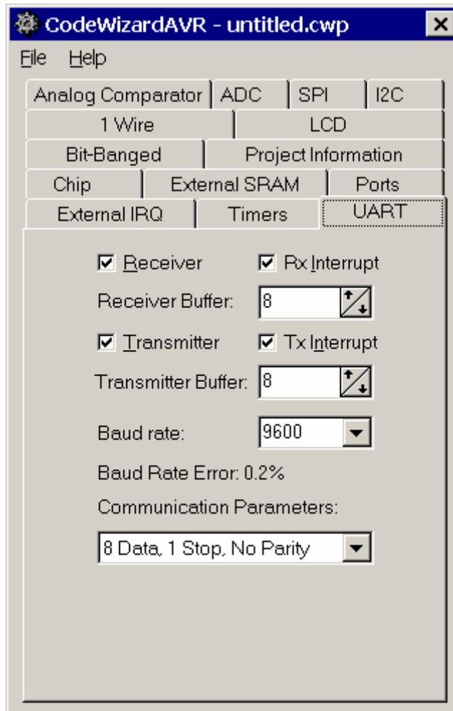
Checking the **Receiver** check box activates the UART receiver.
