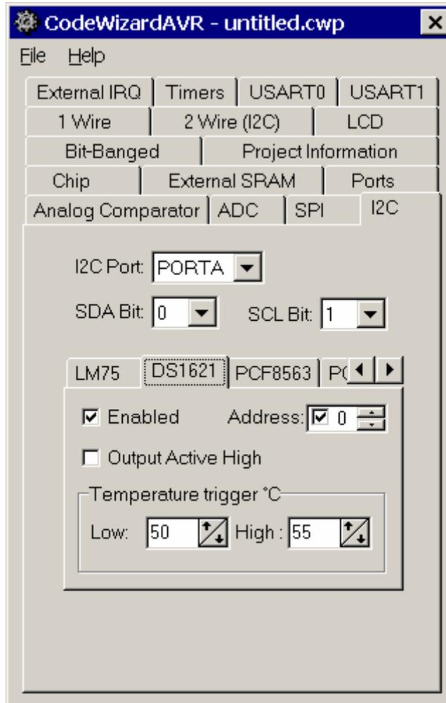
The **Output Active High** check box specifies the active state of the DS1621 Tout output. The **Low**, respectively **High**, spinedit boxes specify the low, respectively high temperatures trigger temperatures for the Tout output.
