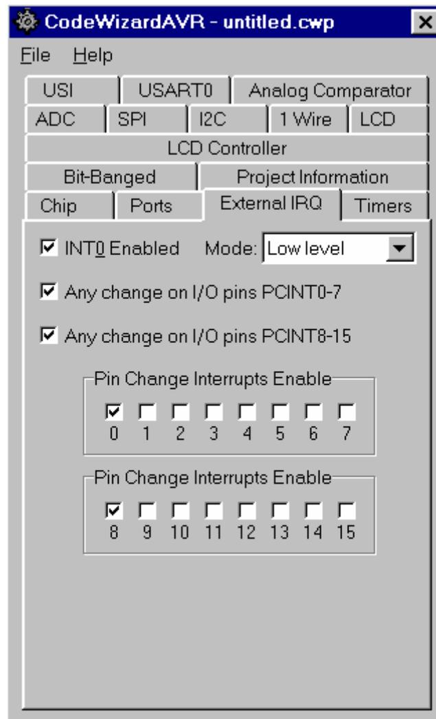
The **Pin Change Interrupt Enable** check boxes, if checked, will specify which of the PCINT I/O pins will trigger an external interrupt.
