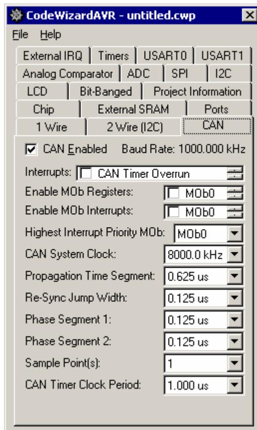
The AVR chip's CAN interface can be enabled by checking the **CAN Enabled** check box. The **Interrupts** list box allows enabling/disabling the following interrupts generated by the CAN controller:
