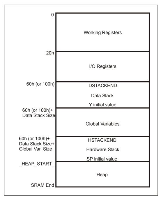
The Working Registers area contains 32x8 bit general purpose working registers.
