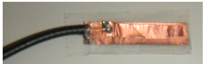
Photo 2. Electrode assembly made from two layers of copper foil and tape.
