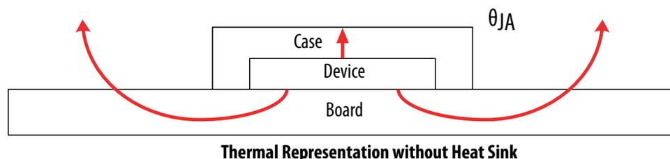
In the model used in the PowerPlay EPE spreadsheet, power is dissipated through the case and board. The  $\theta_{JA}$  values are calculated for differing air flow options accounting for the paths through the case and through the board.
