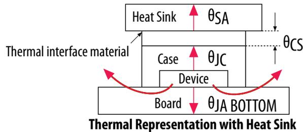
In the model used in the PowerPlay EPE spreadsheet, power is dissipated through the board or through the case and heat sink. The junction-to-board thermal resistance ( $\theta_{JA \text{ BOTTOM}}$ ) refers to the thermal resistance of the path through the board. Junction-to-ambient thermal resistance ( $\theta_{JA \text{ TOP}}$ ) refers to the thermal resistance of the path through the case, thermal interface material, and heat sink.
