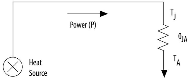
The ambient temperature does not change, but the junction temperature changes depending on the thermal properties; therefore the junction temperature calculation is an iterative process.
