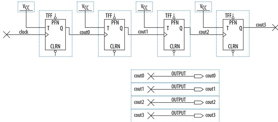
The first TFF with the `cout0` LSB output has a toggle rate of 100% because the signal toggles on every clock cycle. The toggle rate for the second TFF with `cout1` output is 50% because the signal only toggles on every two clock cycles. Consequently, the toggle rate for the third TFF with `cout2` output and fourth TFF with `cout3` output are 25% and 12.5%, respectively. Therefore, the average toggle percentage for this 4-bit counter is  $(100 + 50 + 25 + 12.5)/4 = 46.875\%$ .
