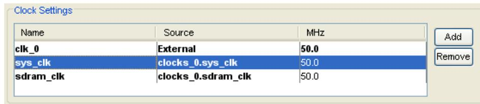
Figure 12. Renaming the system and SDRAM clock.
