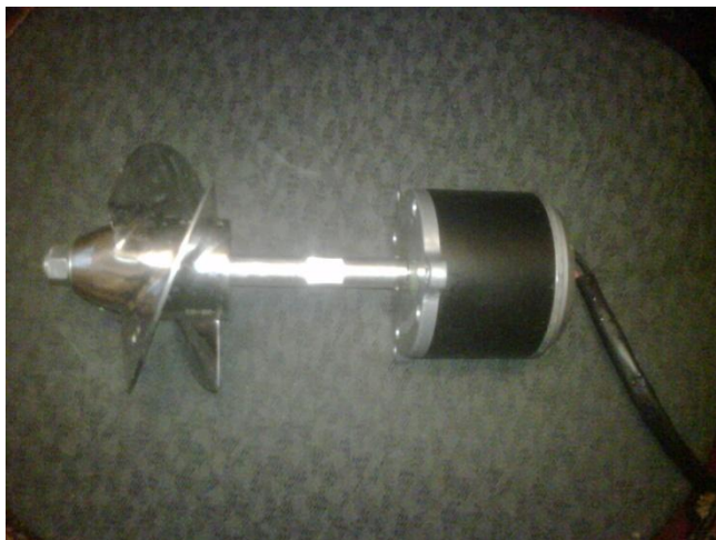
Figure 9: Impeller Connected to Alternator
