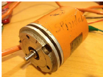
Figure 1. A 1000 ppr Siemens encoder is used as a test piece. The encoder has two phase shifted channels A and B, a marker channel Z and their complements A', B' and Z'. The supply rating is 5VDC.
