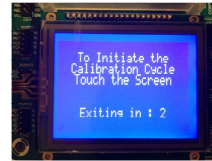
Figure 3. A 128x64 pixel graphics LCD with 4 wire linear resistive touch screen overlay, used as HMI.
