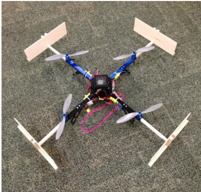
Figure 3: The constructed quadcopter with added pieces to protect the propellers during test flights.
