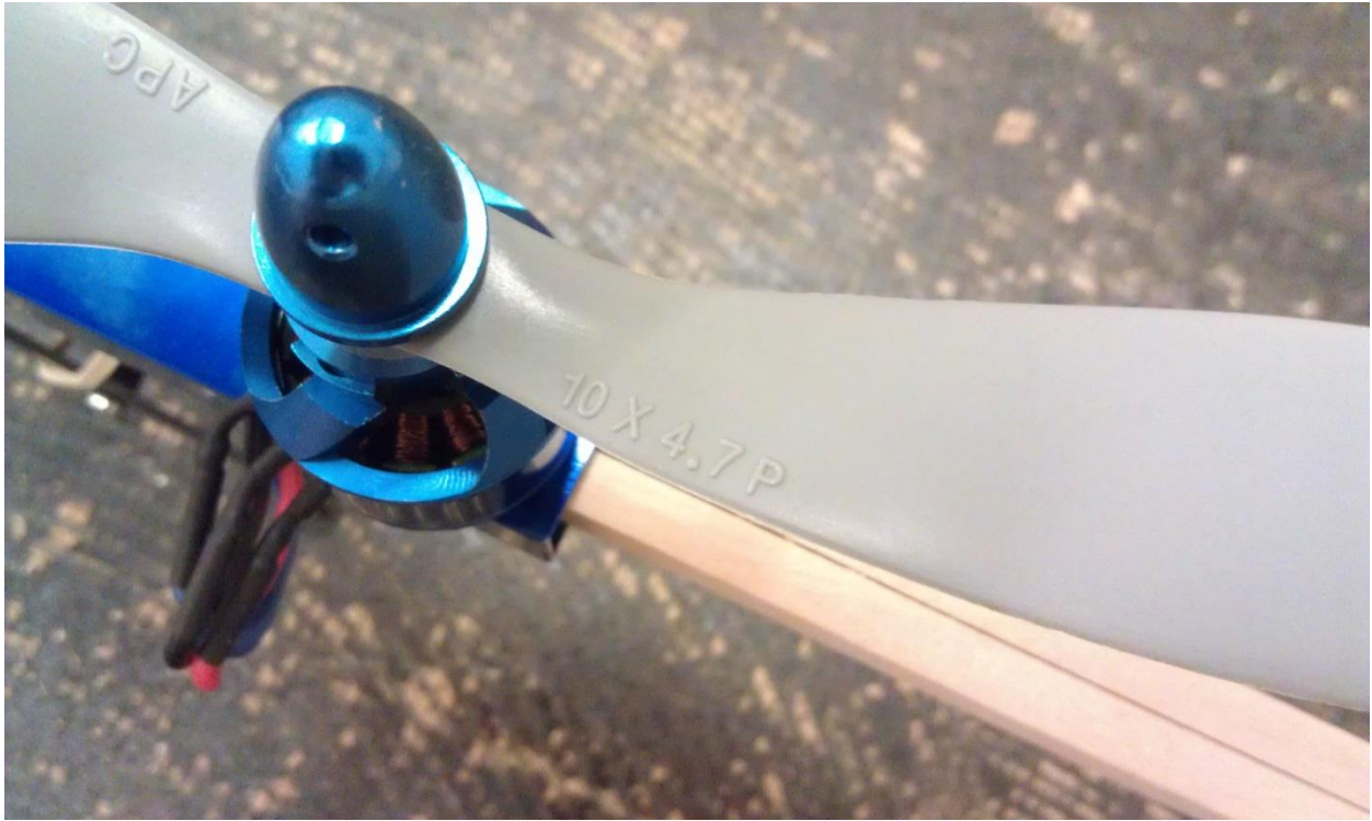
Figure 10: Propeller mounted to brushless motor. Propellers should be mounted with text facing up.
