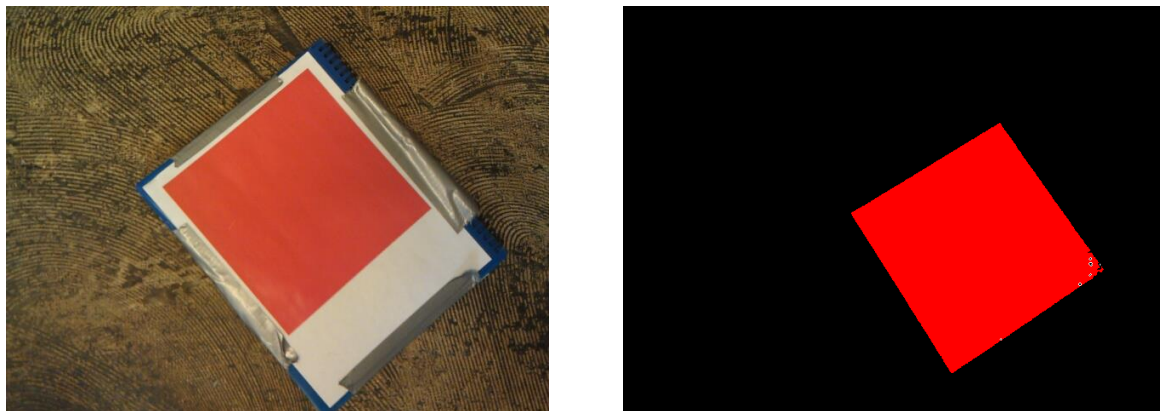
Figure 2: Right: The marker used in this project. Left: The thresholded view of the target used by the algorithm.
