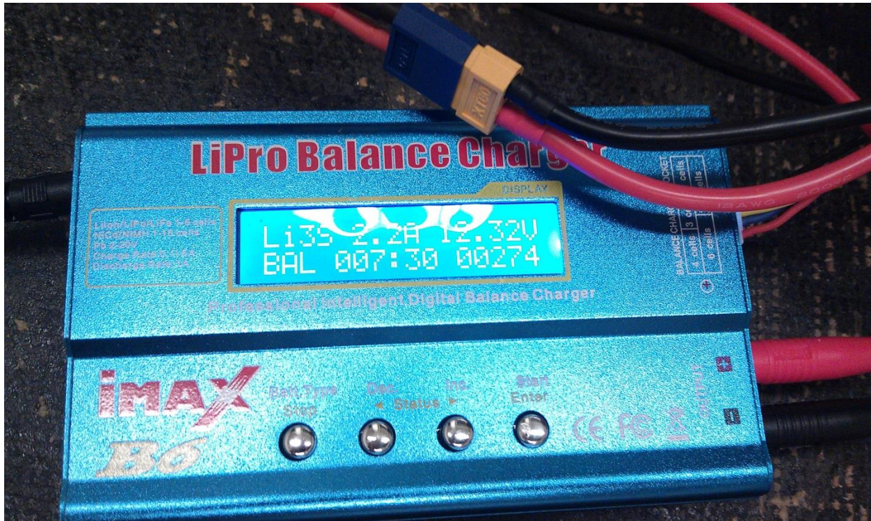
Figure 5: The iMax B6 was chosen because it is affordable battery charger than can balance charge a multicellular Li-Po battery, such as the 3 cell battery that powered the quadcopter.
