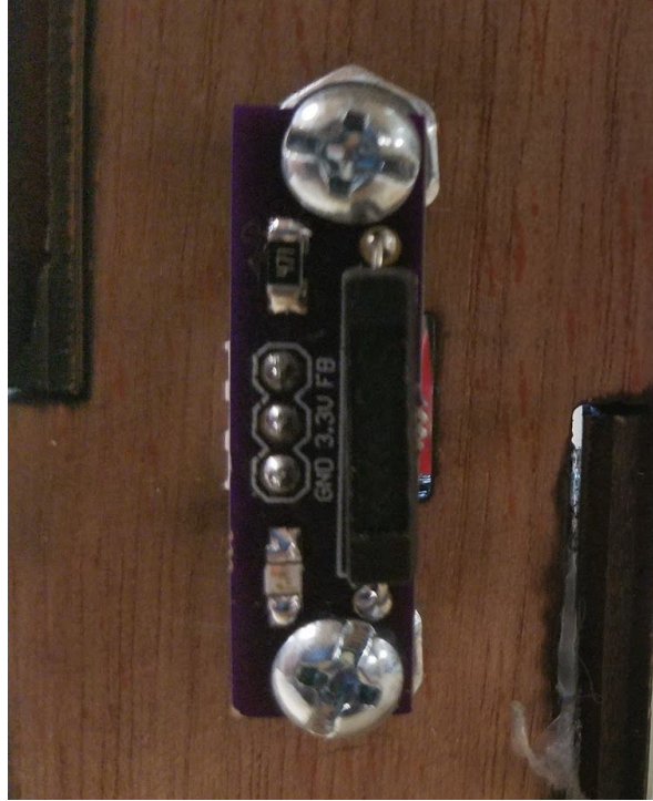
Figure 17: Reed Carrier Mounted to Column
