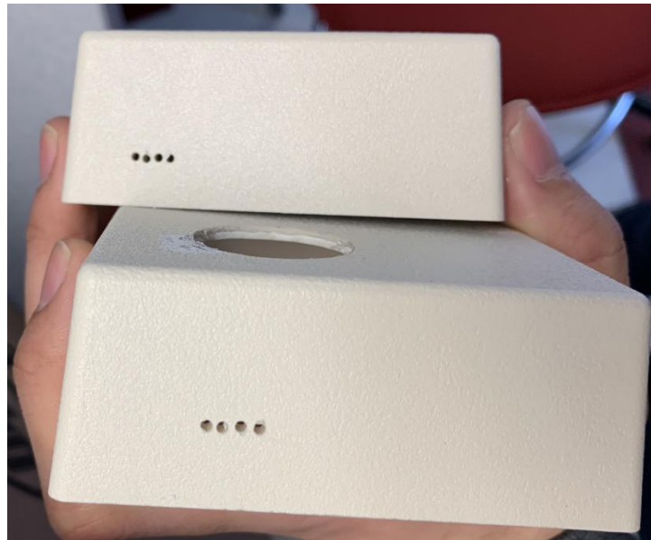
FIG 15 Shape of Hole Drilled by 1mm Drill Bit
