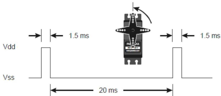
**Figure 11. parallax standard servo timing diagram from data sheet**
