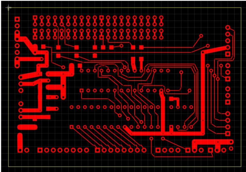
Figure A-4. PIC board Top Layer
