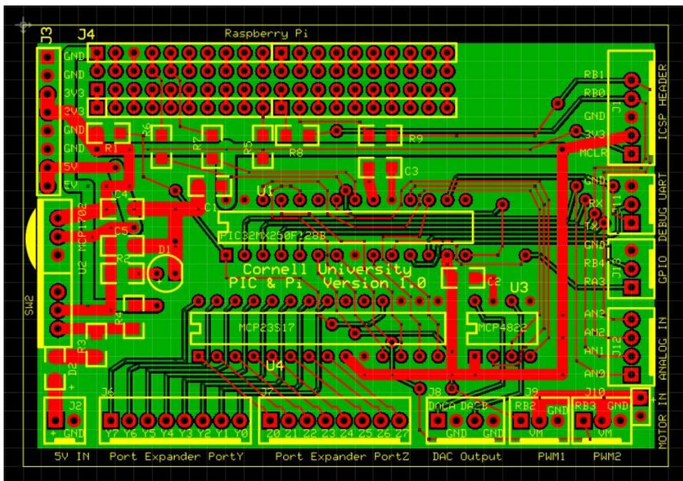
Figure A-3. PIC board PCB Layout
