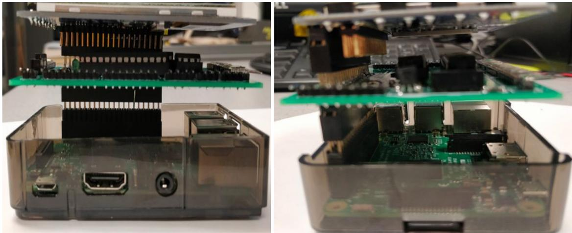
**Figure 15. PIC32 and Raspberry Pi stack side views**
