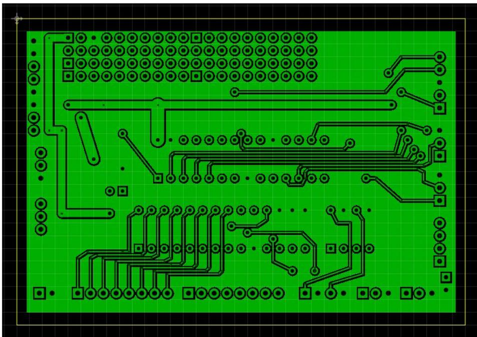
Figure A-5. PIC board Bottom Layer
