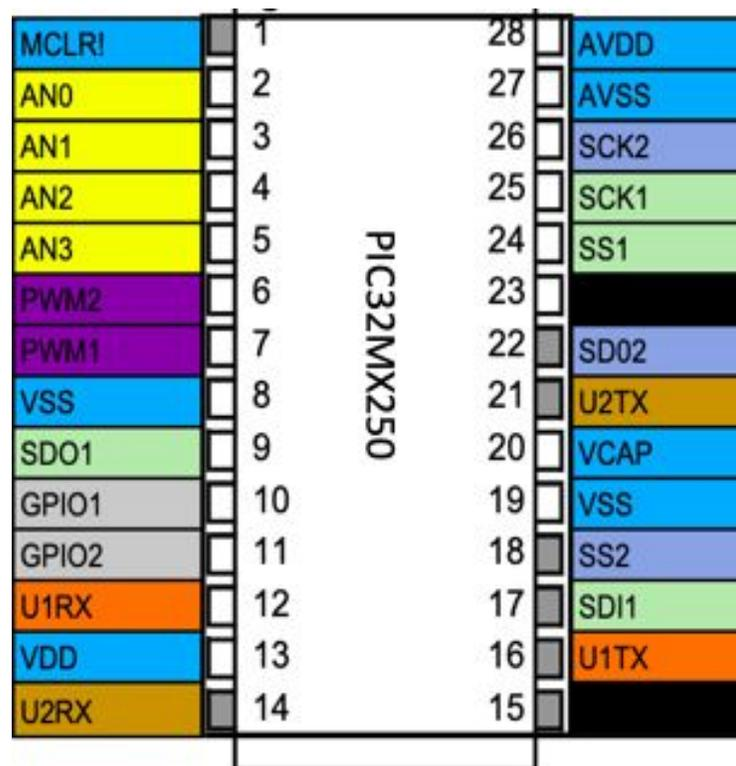
**Figure 2. PIC32MX250 Pin Assignment**
