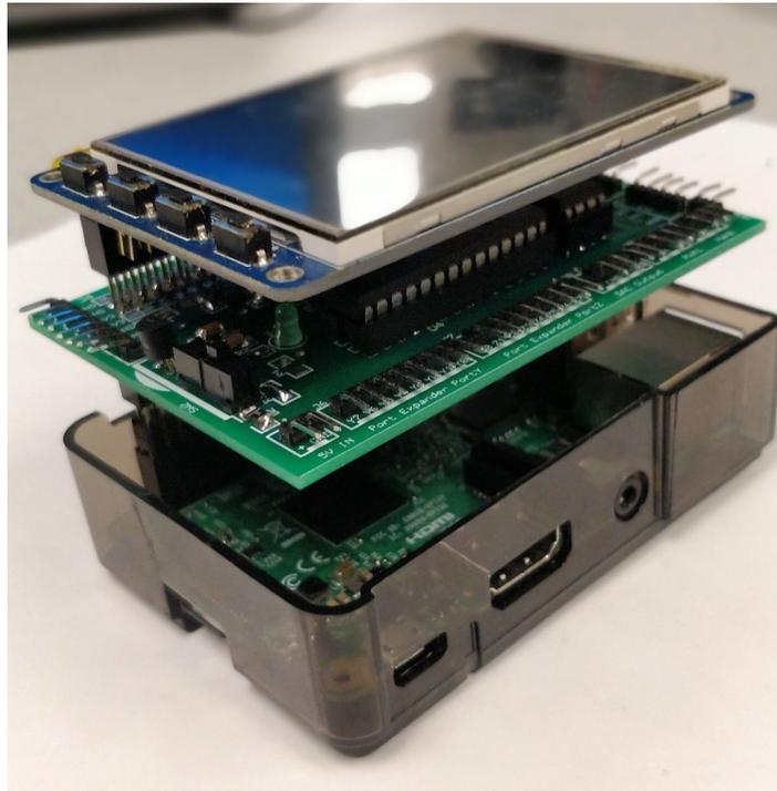
**Figure 16. PIC32 and Raspberry Pi stack**
