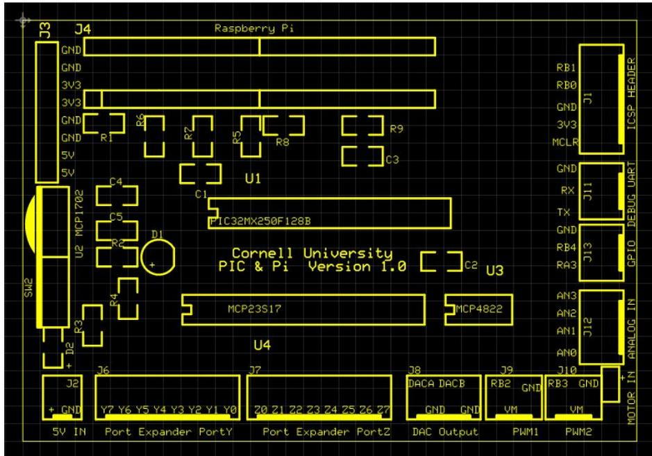
Figure A-2. PIC board General Assembly
