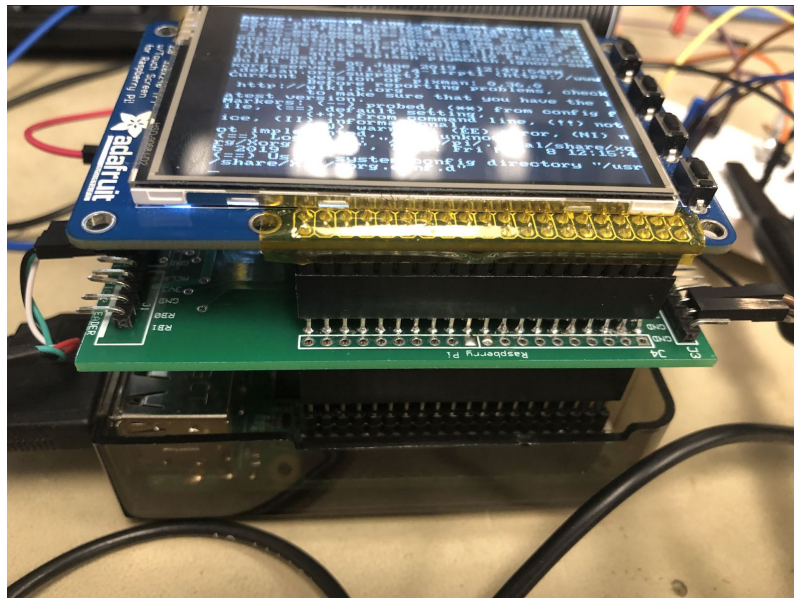
Figure 4. Side view of the raspberry Pi, PIC board and the piTFT stack
